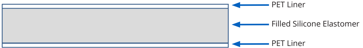
Figure 2. 3M pad 5519 diagram showing PET liners located on top and bottom of the thermally conductive silicone elastomer adhesive layer. The product is available with a conductive layer in thicknesses from 0.5mm to 2.0mm.
