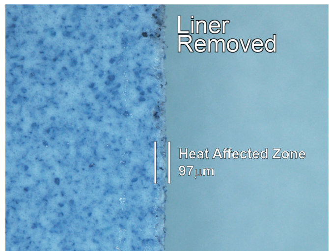
Figure 4. Microscopy image (100X) of the laser-processed edge of 3M pad 5519 with the PET liners removed from the material post-processing. The heat-affected zone measures 97 \mu m.
