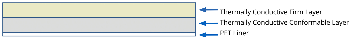
Figure 2. 3M pad 5550H diagram showing PET liners located on the bottom of the thermally conductive acrylate adhesive layers. The product is available in thicknesses of 0.5mm and 1.0mm.
