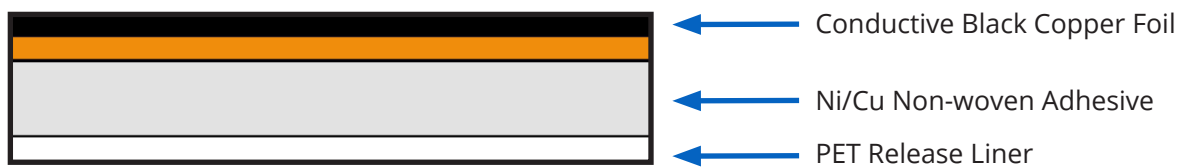
Figure 2. 3M tape 3304BC-S product construction
