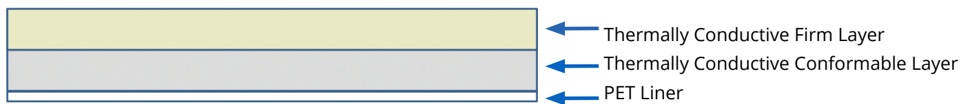
Figure 2. 3M pad 5550H diagram showing PET liners located on the bottom of the thermally conductive acrylate adhesive layers. The product is available in thicknesses of 0.5mm and 1.0mm.
