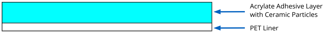
Figure 2. 3M tape 8926-05 diagram showing the thermally conductive acrylate adhesive layer with ceramic particles and PET release liner. The 9826 series tape is available in thicknesses of 0.20mm, 0.25mm, and 0.50mm.
