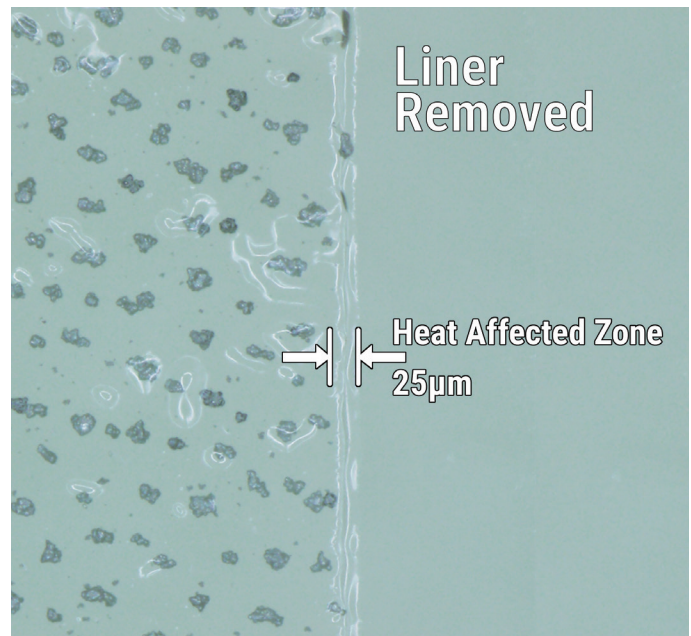
Figure 4. Microscopy image (200X) of the laser-processed edge of 3M tape 9703 with the liner removed from the material post-processing. The heat-affected zone measures 25µm.
