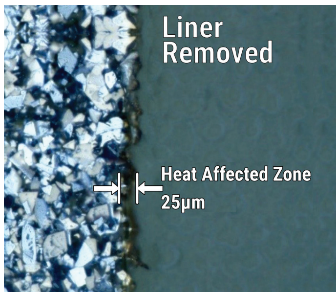
Figure 4. Microscopy image (400X) of the laser-processed edge of 3M tape 9707 with the PET liners removed from the material post-processing. The heat-affected zone measures 25 \mu m.
