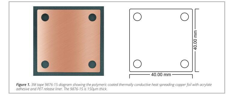
3M<sup>™</sup> Thermally Conductive Heat Spreading Tape applications requiring fine geometry and intricate detail without degrading the physical properties of the material can be achieved with Universal Laser Systems technology. An example demonstrating the results of laser processing the 3M tape 9876-15 material is shown in *Figure 1*.
