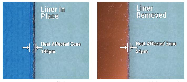
**Figure 3.** Microscopy image (69X) of the laser processed edge of 3M tape 9876-15 with the PET liner in place. The heat-affected zone measures 190µm.
