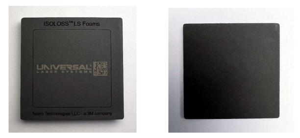
The images above represent top and bottom views of the laser processed ISOLOSS<sup>IM</sup>LS Foam LS-1025. The sample piece demonstrates CO<sub>2</sub> laser cutting (outer edge), scribing (inner square with radius corners), engraving (top and bottom copy), and fiber laser surface marking (logo and DataMatrix code).
