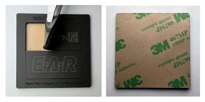
The images above represent top and bottom views of the laser processed ISOLOSS<sup>m</sup> LS Polyurethane Foam LS-1506 and 3M<sup>m</sup> Adhesive Transfer Tape 467MP with 3M<sup>m</sup> Acrylic Adhesive 200MP stack-up. The sample piece demonstrates CO<sub>2</sub> laser cutting (outer edge), kiss-cutting (inner rectangles with top one partially pulled up), engraving (top and bottom text), as well as fiber laser surface marking (logos and DataMatrix code).
