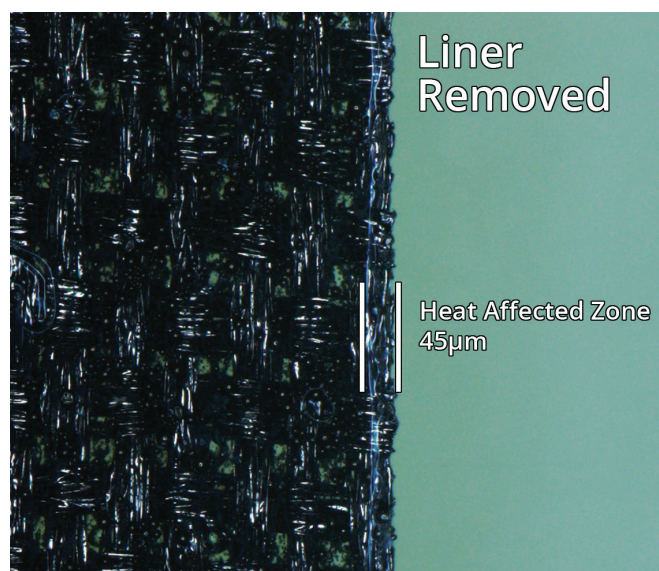
Figure 4. Microscopy image (200X) of the laser-processed edge of 3M tape 9711S with the PET liners removed from the material post-processing. The heat-affected zone measures 45 \mu m.
