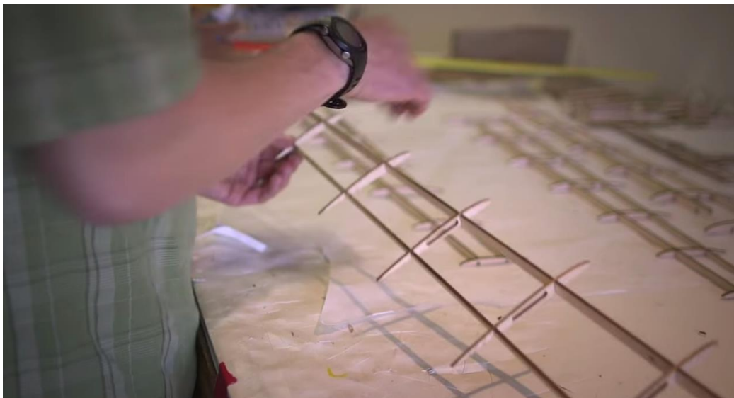
Figure 2. Laser cut components being assembled into a wing structure for an autonomous aircraft.
