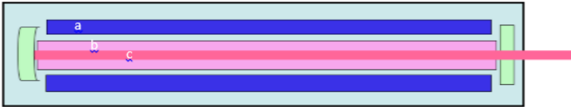
Figure 1. Schematic view of a CO 2 laser showing: a – the RF electrodes, b - the excited CO 2 molecules, c – the laser beam.
