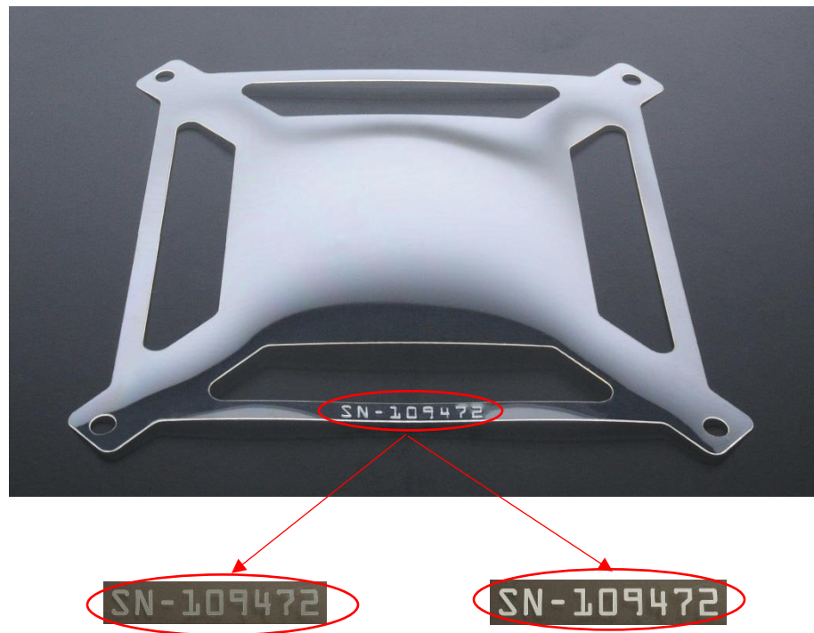
Figure 7. Laser cut PET, with a serial number that was created using a 10.6 \mu\text{m} CO 2 laser (left) and 9.3 \mu\text{m} CO 2 (right).
