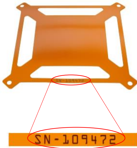
Figure 6. Laser marking on polyimide.
