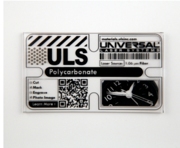
Figure 1: Fiber laser marked sample
